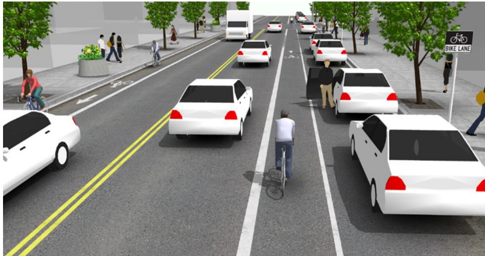
Figure 16: Example cross section of conventional bike lanes
