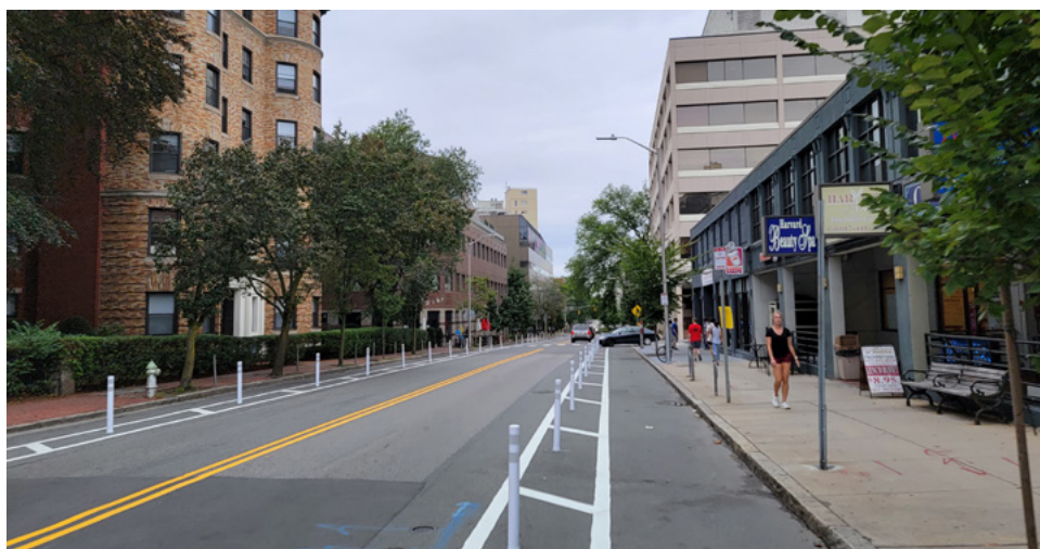
Figure 13: Example of protected bike lanes with gore strip and flex post
