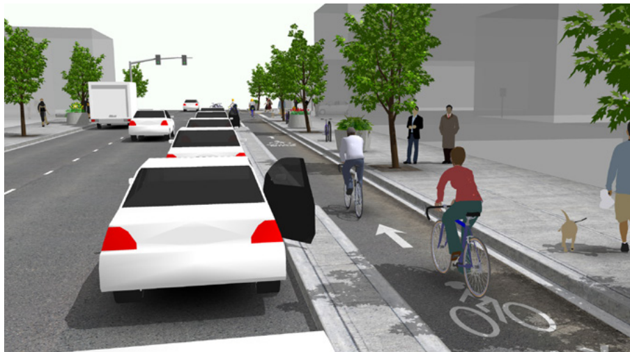
Figure 10: Example of a cross section with protected bike lanes with a curb separation
