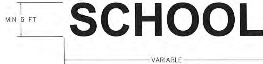
ONE-LANE PAVEMENT MARKING DETAIL
