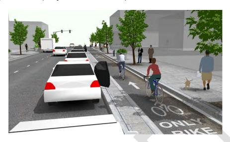
Figure 11: Example of protected bike lanes with parking separation
