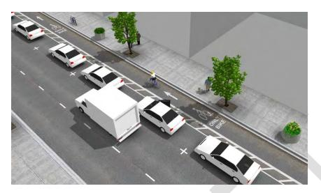
Figure 13: Example of protected bike lanes with gore strip and flex post
