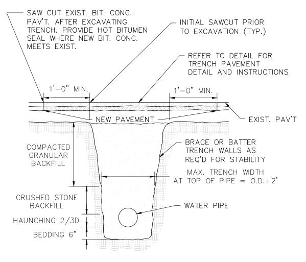
NOTE: DISTRIBUTION MAIN SHALL BE INSTALLED WITH A MINIMUM OF 5' OF COVER.
