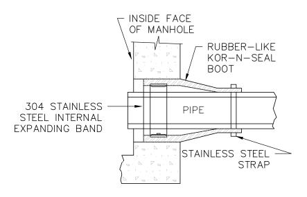
NOTE: KOR-N-SEAL JOINT SLEEVE OR EQUAL
