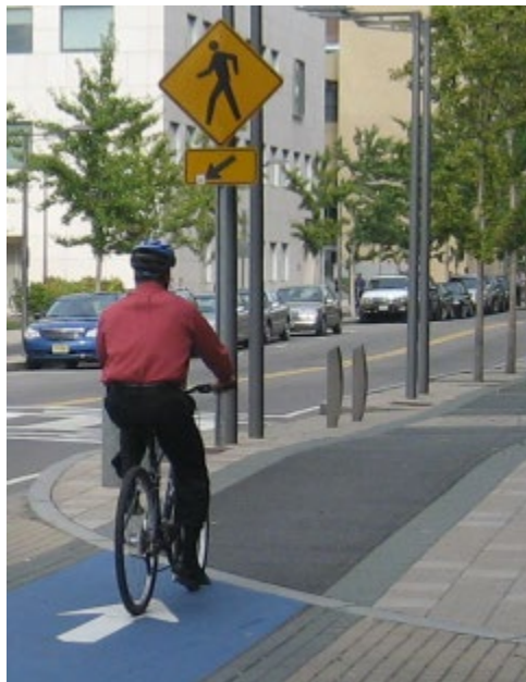
Figure 9: Example of a protected bike lane with curb separation
