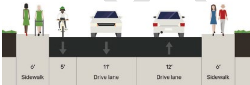
Figure 18: Example cross section of a one-way bike lane
