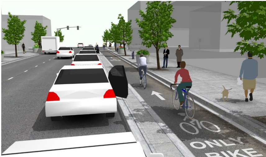
Figure 10: Example of a cross section with protected bike lanes with a curb separation
