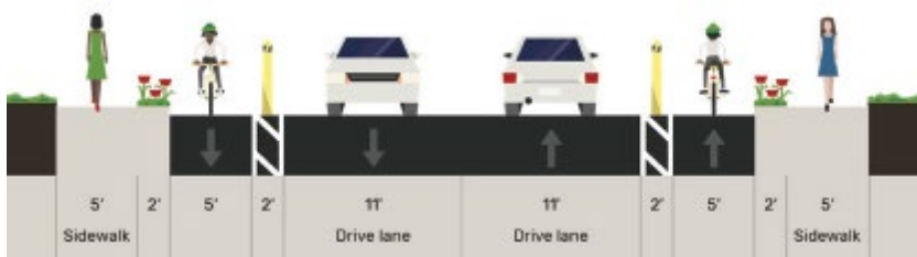
Figure 14: Example cross section of protected bike lanes with gore strips and flex posts
