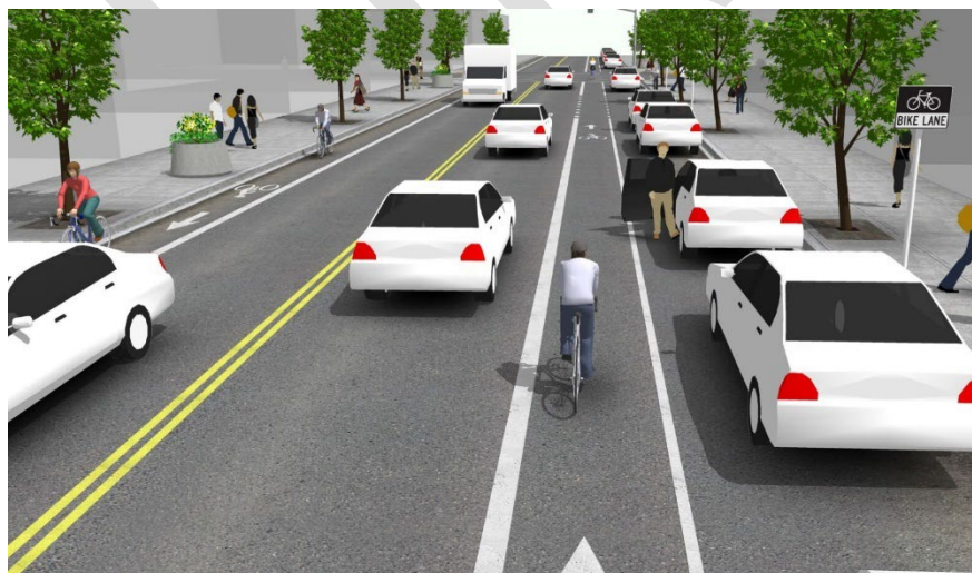
Figure 16: Example cross section of conventional bike lanes
