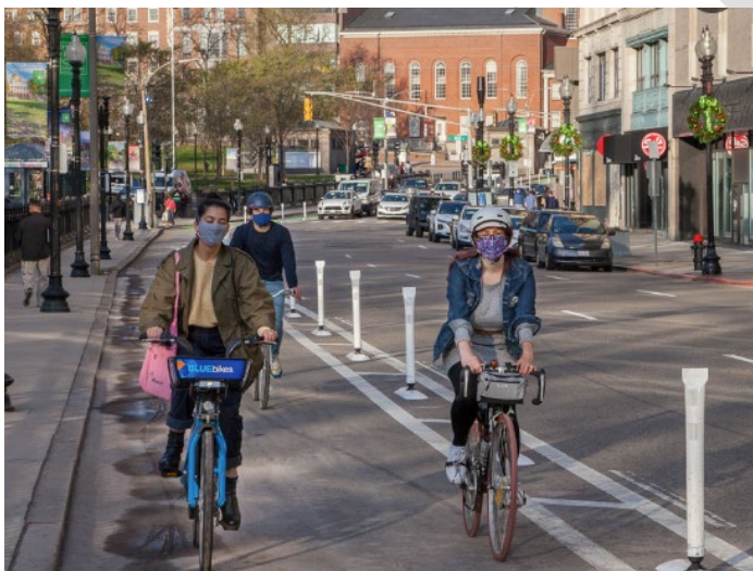
Figure 13: Example of protected bike lanes with gore strip and flex post
