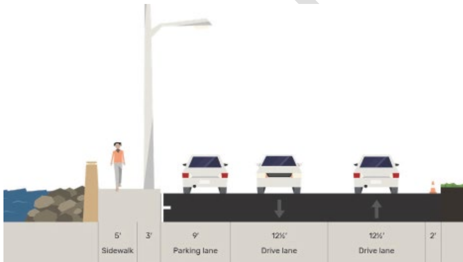
Figure 31: Main Street (Lake Quannapowitt) current cross section
