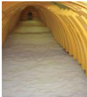
Uniform sediment distribution (US Silica OK-110 SG=2.65).
