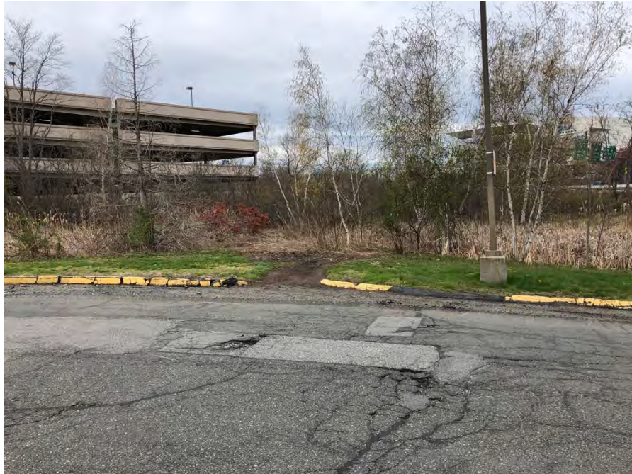
Photo 8: A view of the southwestern corner of Quannapowitt Parkway. Untreated stormwater runoff from the parking lots and roadway discharge into the upland buffer zone before flowing into the BVW in the background of the photo. The stormwater runoff has eroded the uplands buffer zone and is causing sedimentation of the wetlands. The perennial stream is located within the BVW, in the center left portion of the photo.
