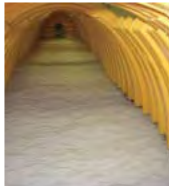
Uniform sediment distribution (US Silica OK-110 SG=2.65).
